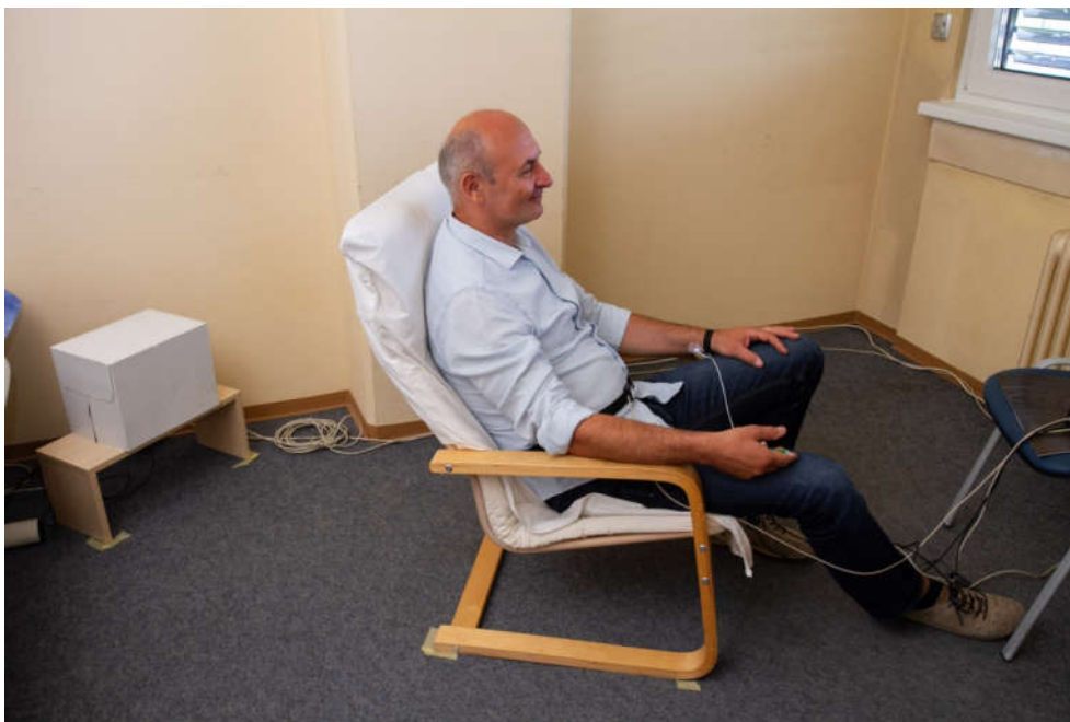
Figure 2: Test setup during testing the supposed protective influence on the human organism against wireless router radiation of the BD PROTECT EMF+ Protection Bracelet. After all the electrodes were attached to a volunteer, he/she sat for 30 minutes while electrophysiological parameters were measured. During the measurements, the Wifi router was hidden under the cardboard box so that neither the test assistant nor the volunteer knew which situation is being tested at a particular time.
